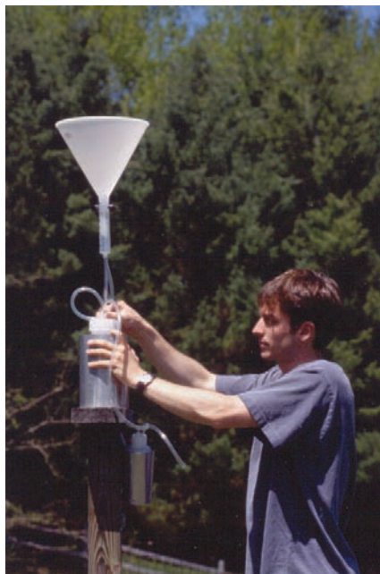
Sampling precipitation chemistry. Photograph: Hubbard Brook Research Foundation Archives
