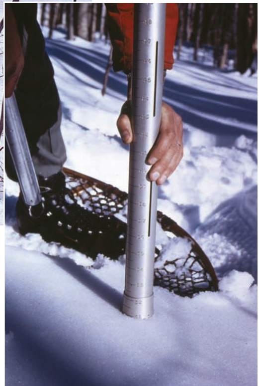
Snow cores are collected and weighed to measure the water content of snow. Photographs: U.S. Forest Service Archives
